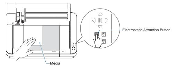
**4.** Make sure that the Electrostatic Attraction Button (white) lights up and the electrostatic adsorption is working before using.
