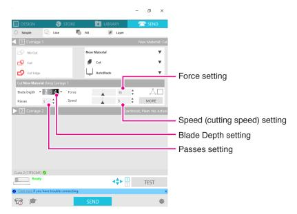
Blade Depth: Automatically protrudes the blade by the amount specified at the time of cutting. (Auto Blade
