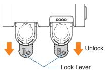
Align the rib of the tool (Auto Blade) with the notch of the Tool Holder and insert it firmly.
