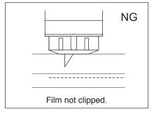
The most important setting in cutting is to adjust the Blade Depth. Adjust so that the blade protrudes slightly more than the thickness of the media to be cut.
