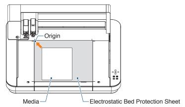
**3.** Lightly fasten the media and press the Electrostatic Attraction Button. The media is fixed by electrostatic adsorption.
