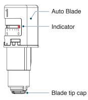
2. Align the recessed part of the Auto Blade tip cap with the protruding part of the handheld blade adjuster and fit it.
