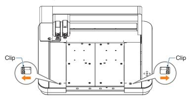
Slide the Electrostatic Bed all the way in and lock it after pushing the clip inward.
