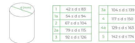
For example, to process a material of **diameter 90 mm** in roller mode, you can place the baseplate at **level 2** and then place the rotary attachment and material for processing.
