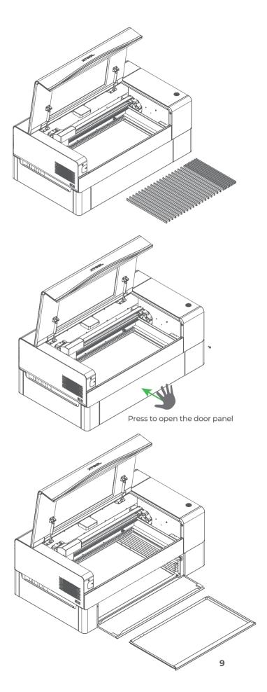
You can keep the removed screw and slats, for subsequent use, in the storage space on the right side of the riser base.
