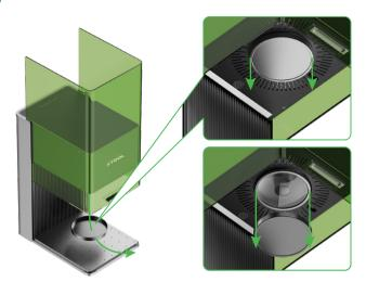
If you won't use the machine for a long period of time, you can install the protector back to prevent the field lens from getting dusty. Ensure that the protector is removed every time before you use the machine.
