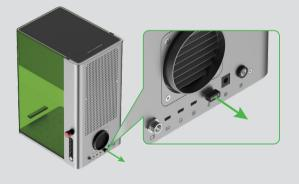
3 Ensure that the emergency stop switch is released. If it is pressed, rotate to release it.
