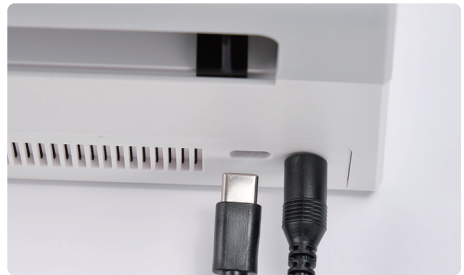
4. Connect the Type-C cable to the printer. (Skip this step for Bluetooth connection)
